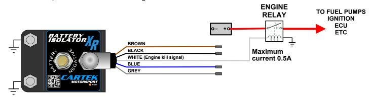
WARNING: The Battery Isolator must be fully connected before starting the engine. If the engine kill output signal is not connected when the engine is running then damage to the Battery Isolator may occur. (Cars without alternators do not apply).
